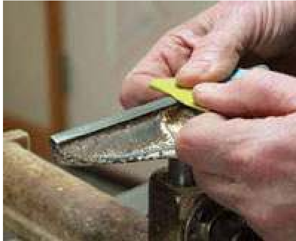
Tune up your tool rest by regularly filing (top) and then sanding (bottom) the surface.
