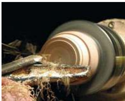
Set your tool-rest height slightly below center with the tool on center.
