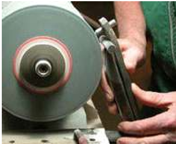
Regular use of a wheel dresser will true your wheel and expose fresh grinding surfaces.
