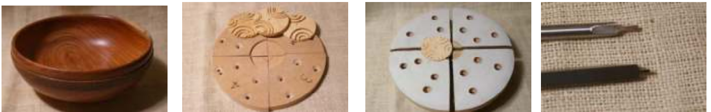
Bill Shean: Blackwood bowl with textured rim, 2 x jigs for cole jaws for offset pieces, tools for same
