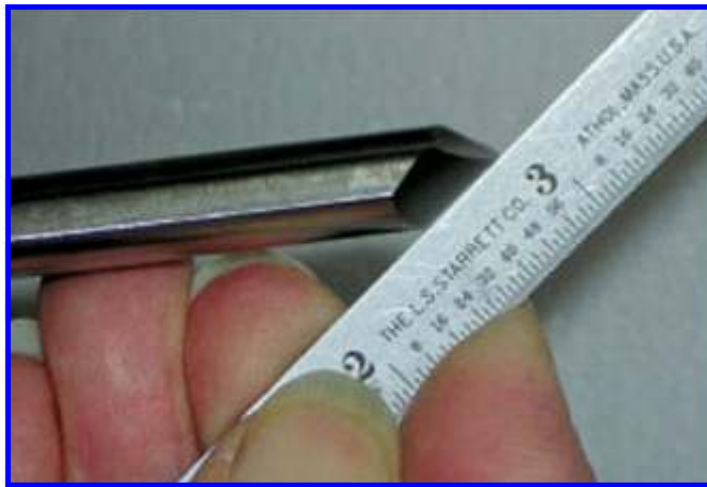
The bevel (grind) of a cutting tool should be flat
