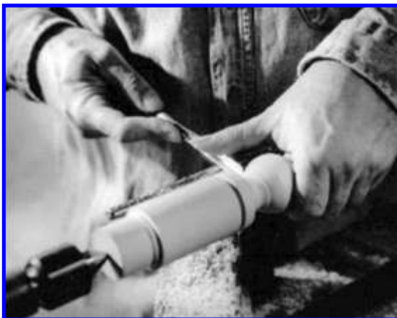
Using the hand to steady vibration
