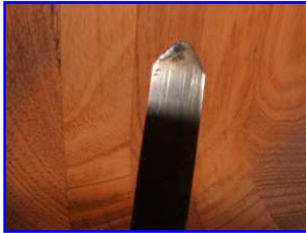
(Photo 13/14) It gives you a very fine planer cut, to promote less use of sanding. (Photo 15)
