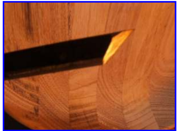
(Photo 13/14) It gives you a very fine planer cut, to promote less use of sanding. (Photo 15)
