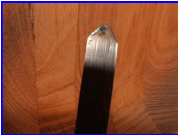
(Photo 13/14) It gives you a very fine planer cut, to promote less use of sanding. (Photo 15)
