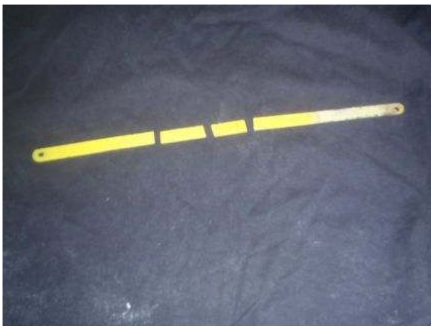
Shattered hacksaw blade that nearly cost me an eye. One of the short middle pieces hit my eye.
