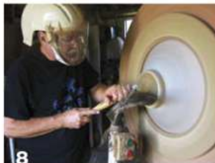
8 At his studio in Hawaii, AAW member Kelly Dunn details the bottom of a bowl with a homemade 36"-diameter Straka chuck on his bowl lathe.
