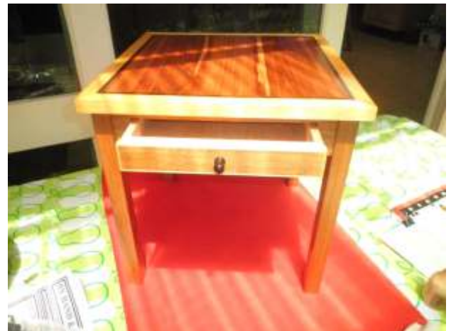
Chris's Bedside Table Made From H/Wood Flooring, Indian Pine and Huon Pine.
