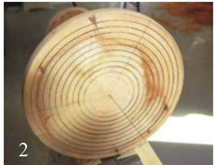
2 Draw lines about every 1/2". Cut into these lines lightly with the long point of a skew or corner of a parting tool. Divide the disc into three equally spaced sectors.
