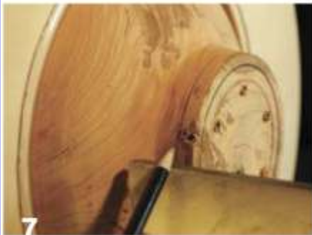
7 To center the piece on the chuck, use a pencil to find the high point of the bowl. Loosen the wing nuts, push from the center of the penciled length, and tighten the nuts.
