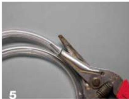
To pad a ring with clear plastic hosing, cut through the top of the natural curve of the hose. When cut like this, the natural spring of the hose will hold it inside the opening.
