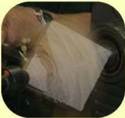
Simply jamb the square block of timber between centres.....
