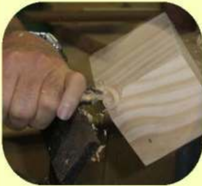
Mount the block in the chuck and start turning the base.....
