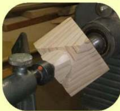
Using a parting tool to shape a spigot for the chuck.....
