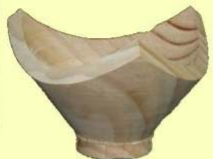
Reverse chuck the blank and your ready to start on the inside.....
