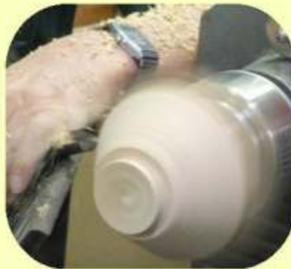
Shape the outside of the bowl until you reach the desired effect.....
