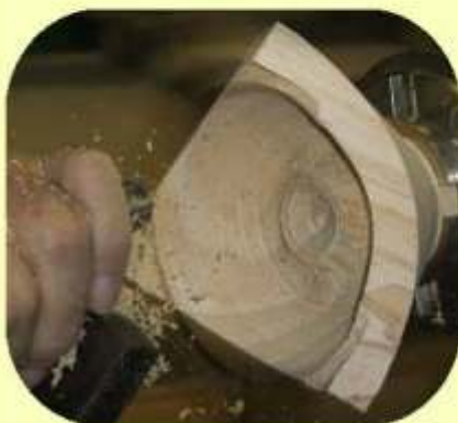
Keep shaping the inside until you reach the desired wall thickness.....
