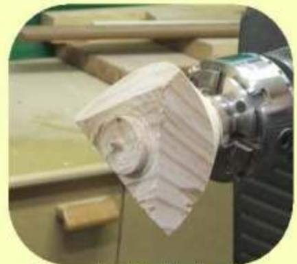
Reverse chuck the blank and your ready to start on the inside.....
