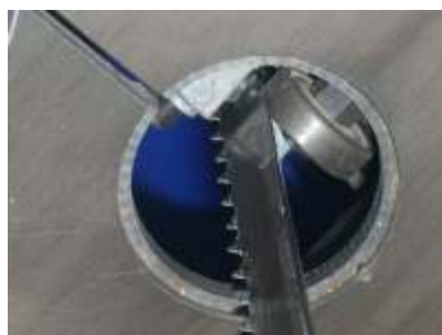
Looking through the table with the plastic insert removed, into the plastic piping
