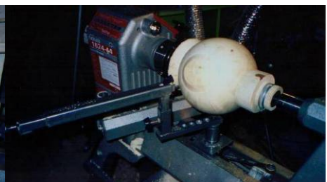
Finish turning the sphere with the ball turner, between cup chucks
