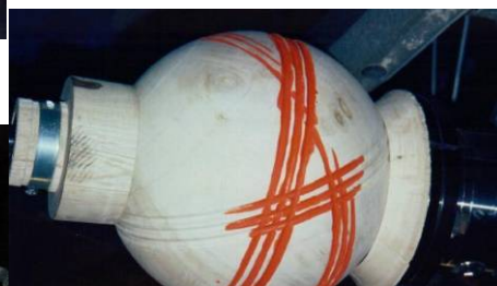
Add colour to the grooves and sand to 400 grit
