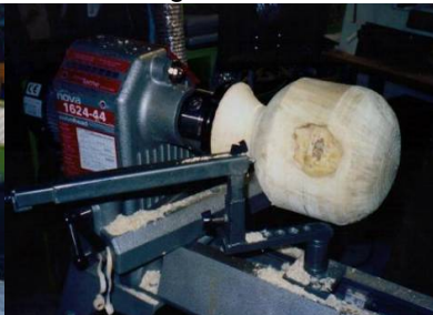
Turning the ball using the adjustable ball turner of the author's design
