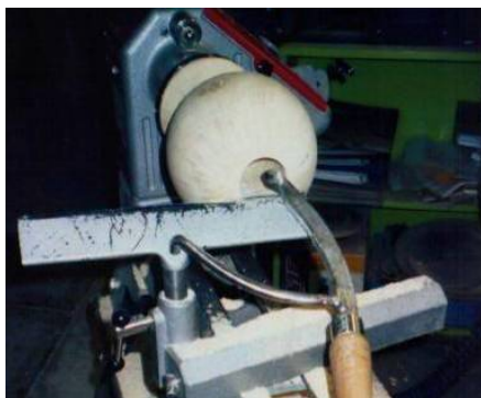
Hollowing out to about 8mm wall thickness
