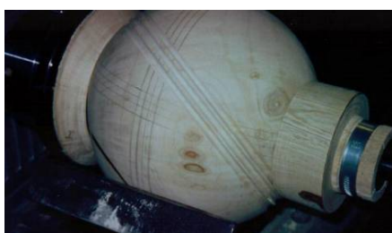
Marking and turning grooves while mounted between cup chucks
