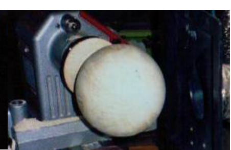
Sand to about 240 grit. Note vacuum suction device on right
