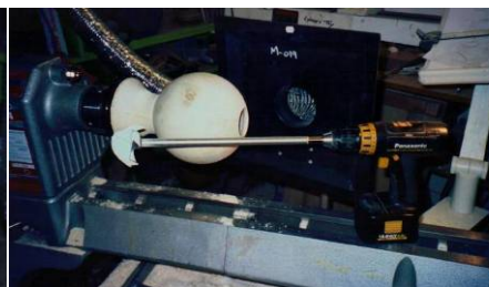
Sanding inside with a homemade extension sander
