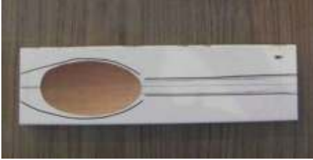
Paul begins by cutting a board to suit the size of the spoon and marking out the shape he wants.
