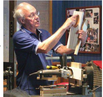
Paul begins by cutting a board to suit the size of the spoon and marking out the shape he wants.
