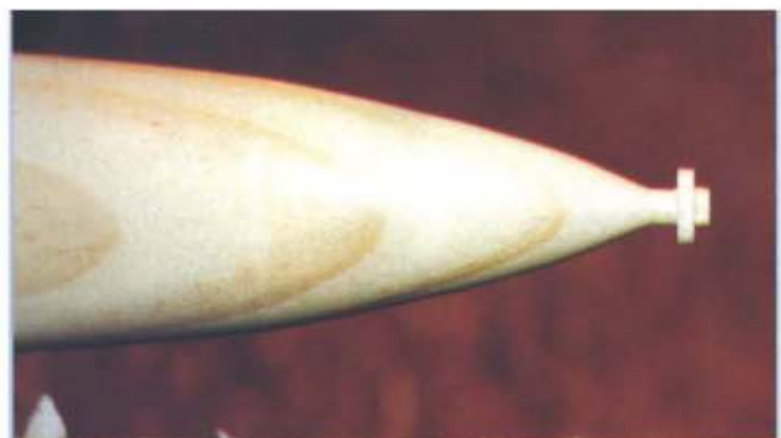
Photo 2: The cross is turned and later sanded flat on two sides.
