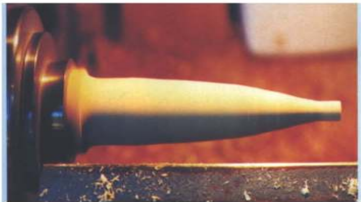
Photo 1: The tree (Radiata Pine) is shaped to a gradual taper then turned smooth.
