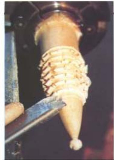
Photo 4: The skew is rolled anti-clockwise slightly to accentuate the roll
