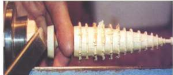
Photo 6: The base is undercut to ensure the tree sits firmly on the rim.
