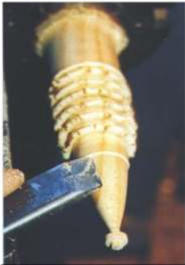
Photo 3: Each branch is created by cutting uphill with the long point of the skew
