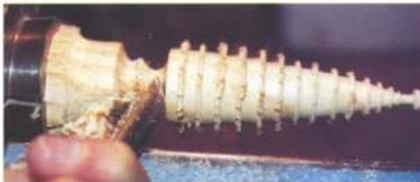
Photo 5: The trunk may be turned with either a gouge or a scraper.
