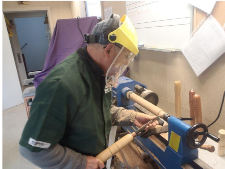
ME WORKING ON A TURNING A TOOL HANDLE.
