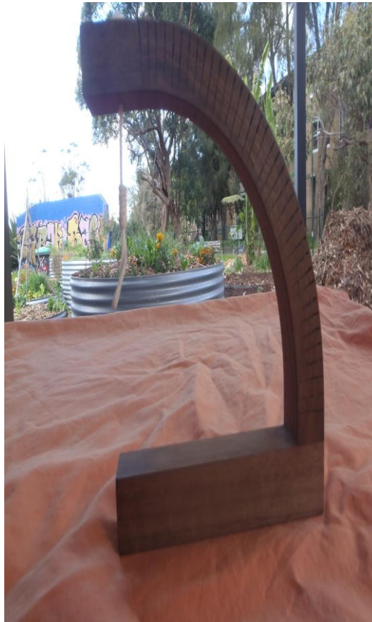
ARCH MADE USING SAW KERTFING.
